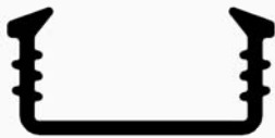
AU3224 – 'U' Channel. Please see Aluminium Gaskets & Pressure Plates for complete range. (Scale 1:1)
